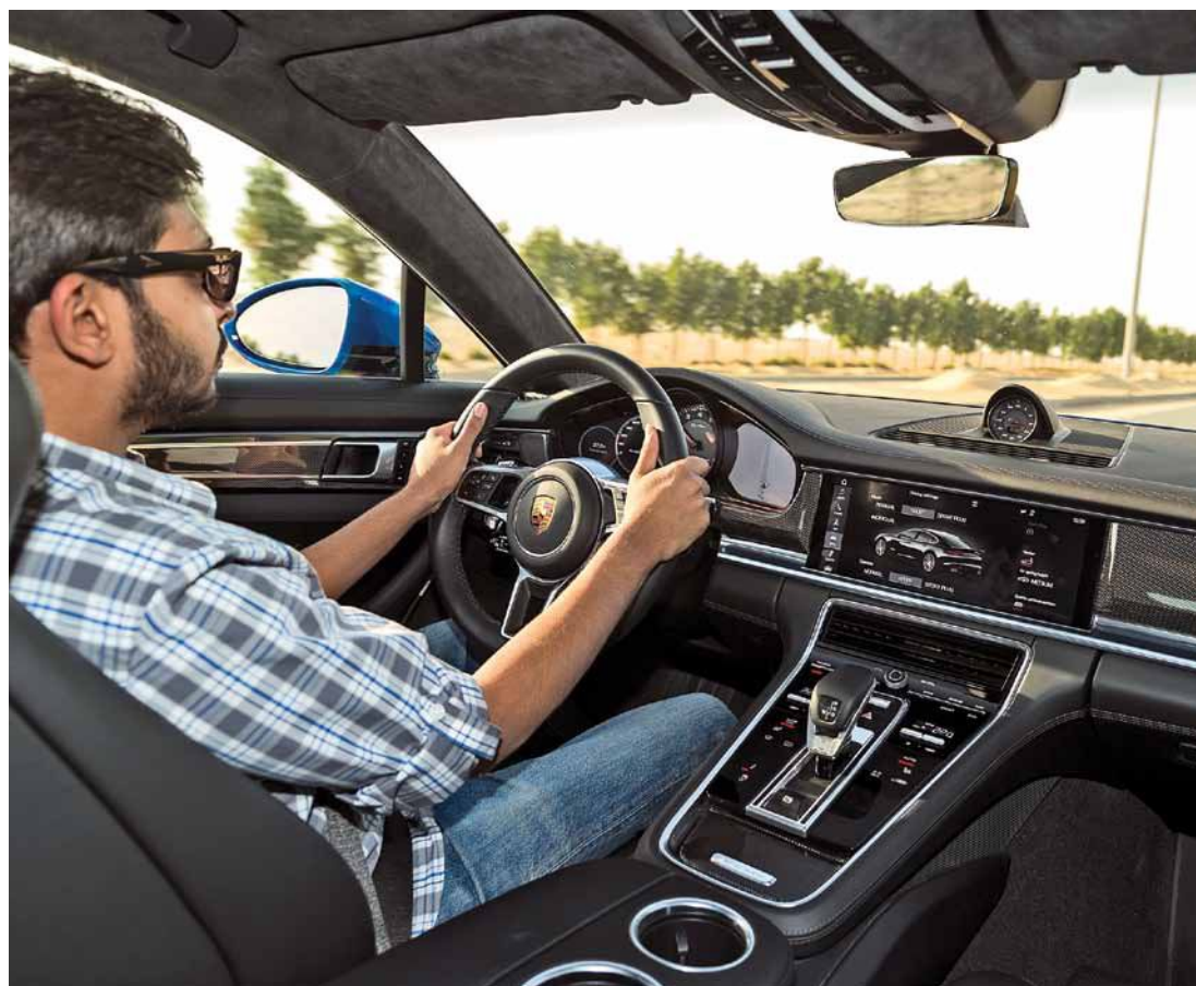
Small knob on the steering wheel lets you switch between different drive modes
