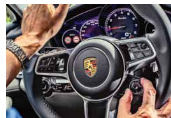
Small knob on the steering wheel lets you switch between different drive modes
